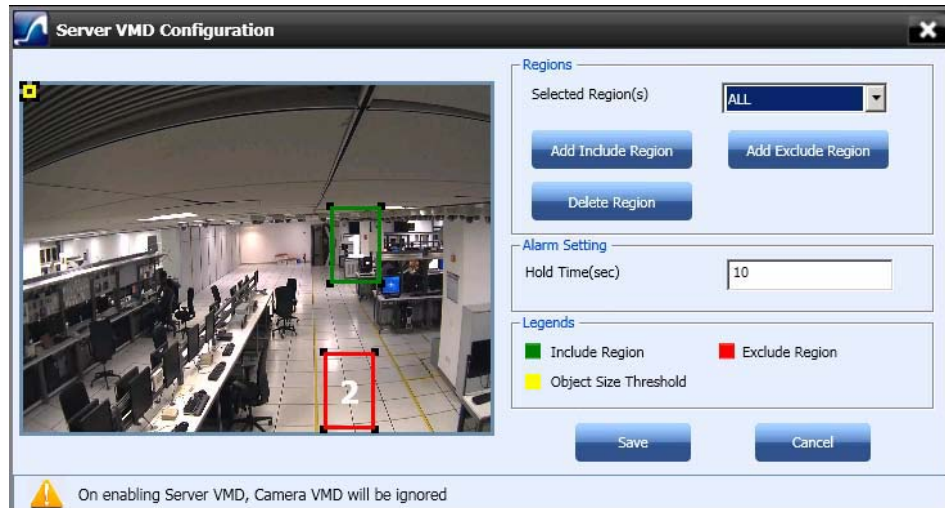
Figure 4-17 Server VMD Configuration
