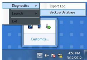
**Figure 3-20** Taking Database backup using the MAXPRO NVR Agent
