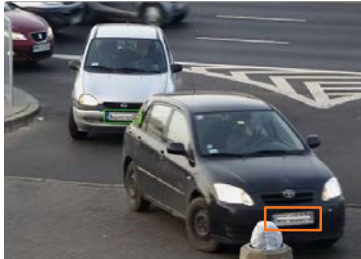
Depth of field is insufficient to cover foreground license plates. Adjust the lens settings.
