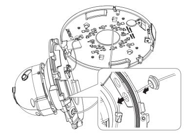
4-4. Connect the network cable jack to the PoE+ port of the camera.
