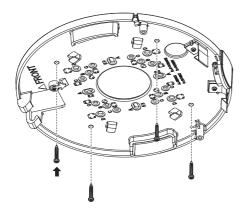
1-3. Pull out necessary cables among network/power/audio/alarm cables through the hole in the mount plate.
