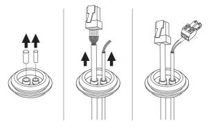
3-4. Mount the cable bushing to the camera body.
