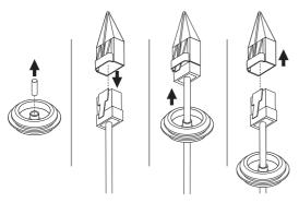
4-3. Mount the cable bushing to the camera body.
