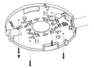
2-5. Pull out necessary cables among network/power/audio/alarm cables through the pipe.
