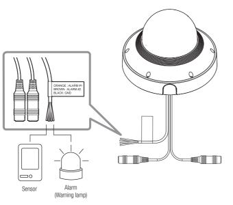
ALARM #1, ALARM #2 : These ports can be used as alarm input or output ports. If used as input ports, alarm input or day/night sensors can be connect to them. If used as output ports, alarm output signals can be connect to them.
