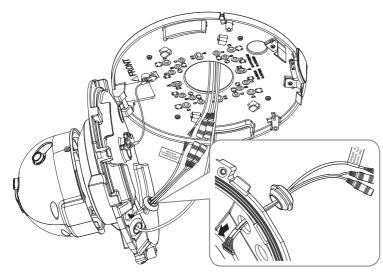
6. Connect the connector of the audio/alarm cable to its connection port.
