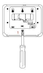
With a small phillips screwdriver, undo the locking screw from the back of the panel and remove the SmartMount backplate.
