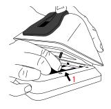
1. Locate the IQ Base with SmartMount and connect the power cable from the IQ Base into the BLACK connector inside the IQ Panel 4. Refer to Interior Diagram on Page 7
