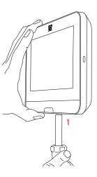
1. With a small phillips screwdriver, screw in the locking screw from the bottom of the panel to secure it to the wall.
