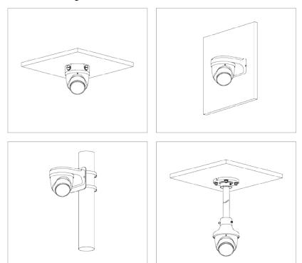
Figure 3-4 Installation methods
