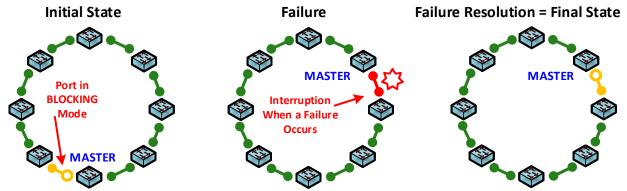
$\square$  The switchover time to the back-up line is for LAN-RING protocols slightly dependent on the number of switches connected in the ring. With each switch connected to the ring, the reconfiguration time increases by only about 6µs!
